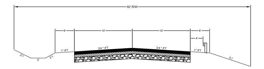
Item 441 - 2" Asphalt Concrete Surface Course, Type 1, (448), (Leveling), (PG 64-22)
